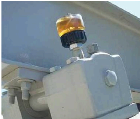
OIL RESERVOIR New improvement to Drake 16 and 25 models
